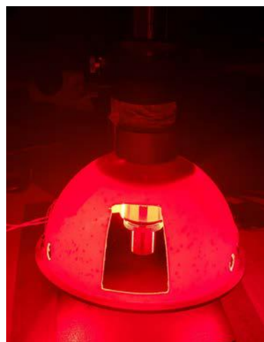
Fig. 2. Upper illuminator with red light diode
