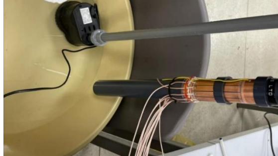
Fig. 2: Typical Test Rig Setup with ECT Sensor N-Electrode.
